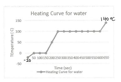
22. Which line segments on the curve show an increase in average kinetic energy? How about an increase in potential energy? Inc. in avg. KE: t=25 to t=50, t=150 to t=250, t=600 to t=650 Inc. in potential energy: t=50 to t=150, t=250 to t=600
